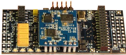
Figure 1. The Chip-EC carrier board ( with no mezzanine)
